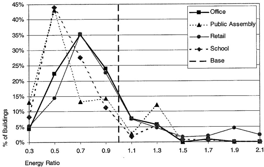
**Figure 5: Lighting Energy Ratio by Building Type**
