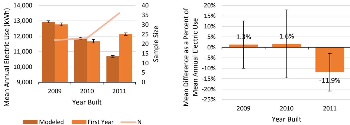
**Figure 7.** Comparison of mean modeled vs. first year normalized electric use (in kWh) and mean differences as a percent of mean annual usage in electric heated EPS homes built from 2009-2011. Note: positive values indicate that models overestimated usage, on average, while negative values indicate that they underestimated it.
