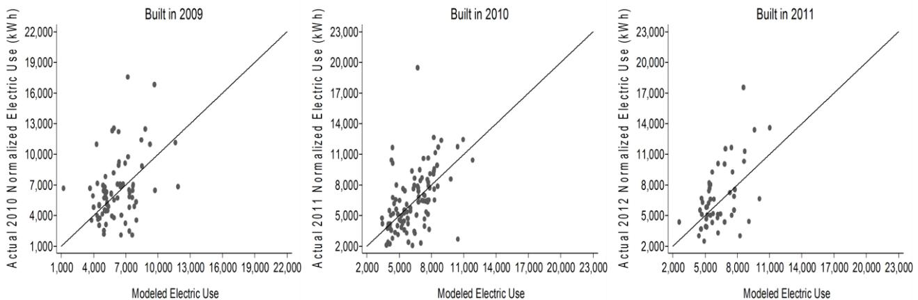
**Figure 4.** Scatterplots of modeled electric usage versus the deviation in first year normalized electric use from modeled usage (in kWh) in gas heated EPS homes built from 2009-2011. Note: the reference line indicates where first year and modeled electric use are equivalent; points above the line indicate homes where actual usage was higher than estimated and vice versa.
