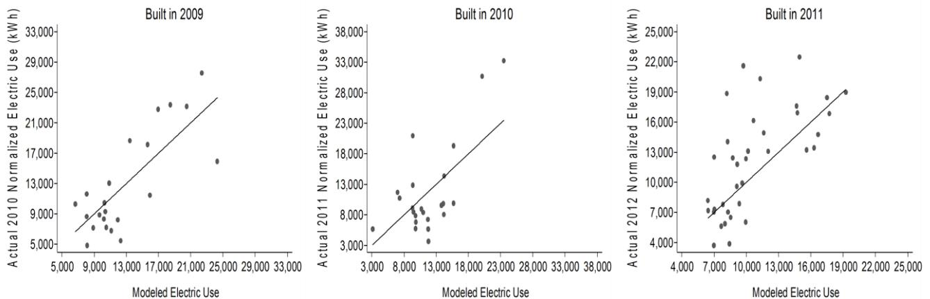
**Figure 8.** Scatterplots of modeled electric usage versus the deviation in first year normalized electric usage from modeled usage in electric heated EPS homes built from 2009-2011. Note: the reference line indicates where first year and modeled electric use are equivalent; points above the line indicate homes where actual usage was higher than estimated and vice versa.
