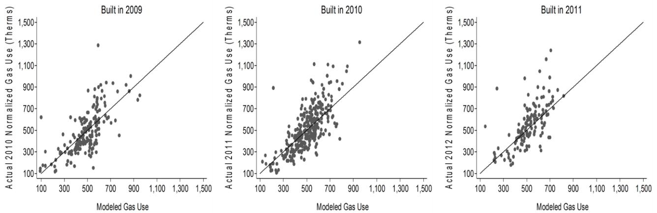
**Figure 2.** Scatterplots of modeled gas usage versus the deviation in first year normalized gas use from modeled usage (in therms) for individual gas heated EPS homes built from 2009-2011. Note: the reference line indicates where first year and modeled gas use are equivalent; points above the line indicate homes where actual usage was higher than estimated and vice versa.
