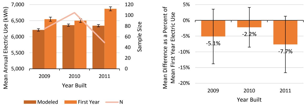
**Figure 3.** Comparison of mean modeled vs. first year normalized electric use (in kWh) and mean differences as a percent of mean annual usage in gas heated EPS homes built from 2009-2011. Note: positive values in the graph of differences indicate that models overestimated usage, on average, while negative values indicate that they underestimated it.
