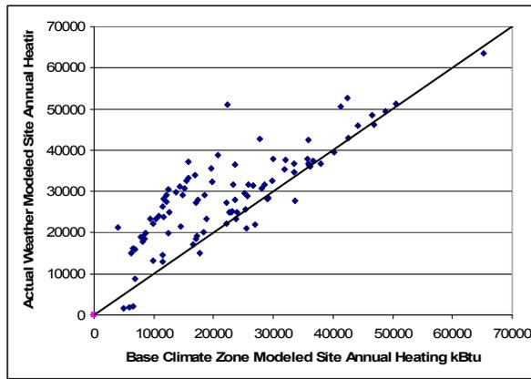
**Figure 4: Single Family Heating Base Weather Results Compared to Real Weather Reruns**
