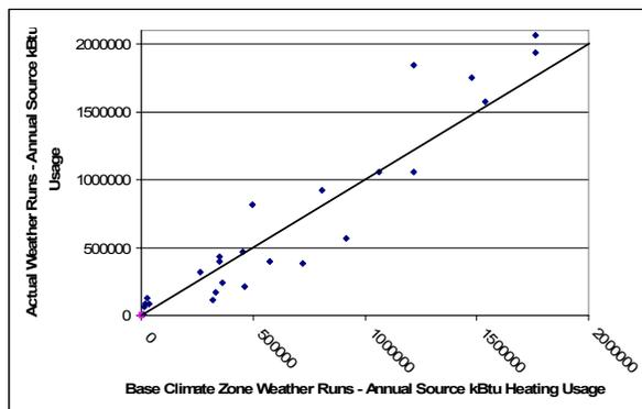
**Figure 5: Multi Family Heating Base Weather Results Compared to Real Weather Reruns**
