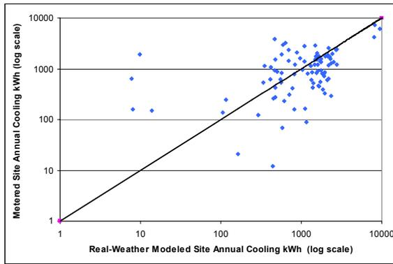
**Figure 6: Single family Metered Annual kWh Cooling Compared to Modeled kWh Cooling, log scale**
