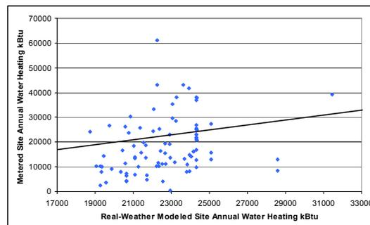
**Figure 8: Single family Metered Annual Water Heating Compared to Modeled Water Heating**
