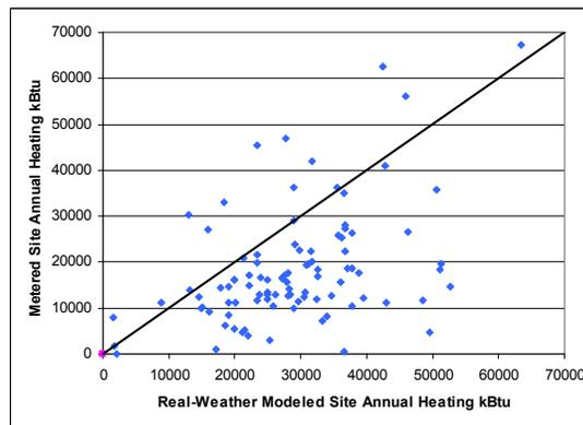
**Figure 7: Single family Metered Annual kBtu Heating Compared to Modeled kBtu Heating**
