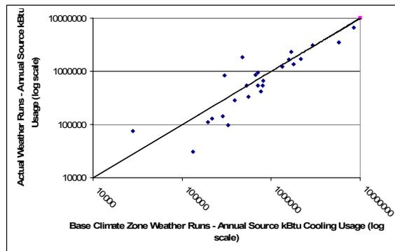
**Figure 3: Multi Family Cooling Base Weather Results Compared to Real Weather Reruns**
