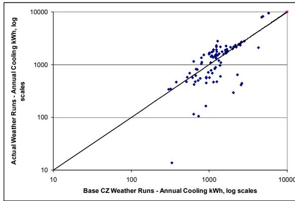
**Figure 2: Single Family Cooling Base Weather Results Compared to Real Weather Reruns**
