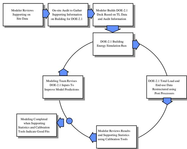
**Figure 2 - Overview of Re-Simulation Approach**
